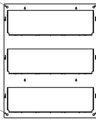
STEP 3. Peel off the protective film on each Divider (B). Slide 1 divider down and insert the tab into the slot on the back panel. Twist the divider and snap it into place.
