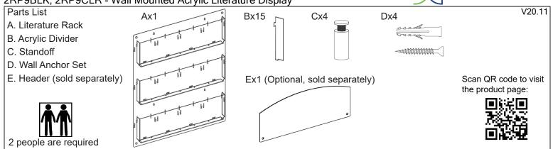
STEP 1. Hold the Literature Rack back panel (A) against the wall at the desired mounting location. Make sure the panel is level and mark the center of each hole.
